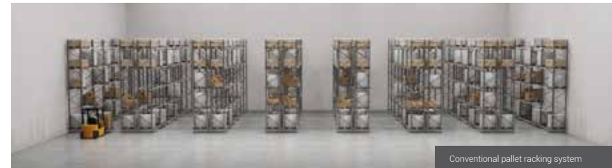
Conventional pallet racking system
